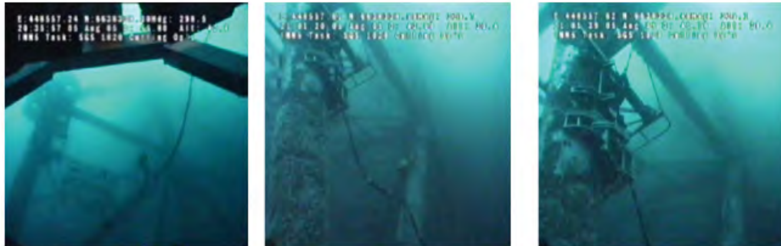
Subsea docking of ROV Flown (DWCT) Cutting Tool
