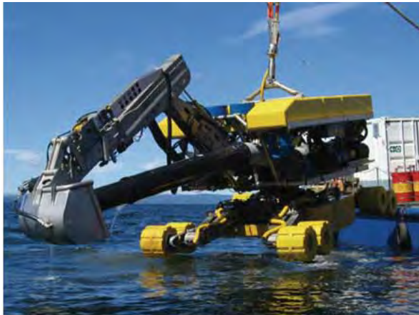
Nexan Spiders cleared a path and dug subsea trenches from Ormen Lange to Nyhamna. (Photo courtesy of Norsk Hydro)
