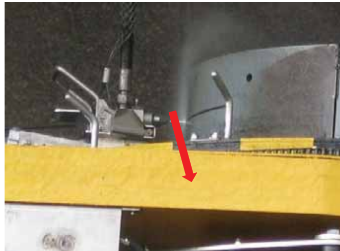
Diamond Wire Cutting System (DWCS)
